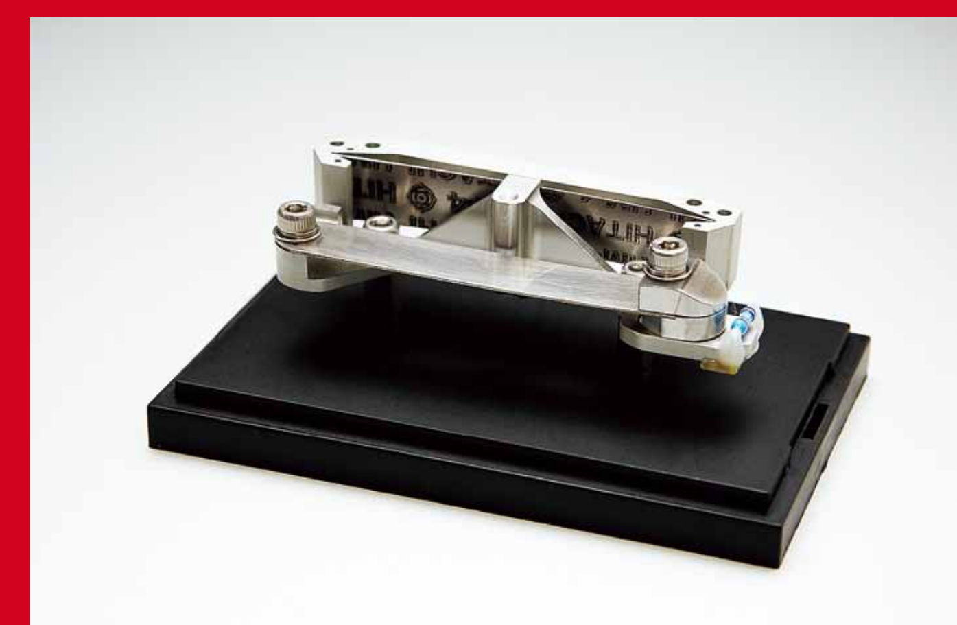
The environment driven mobility system for the asteroid exploration robot onboard Hayabusa-2
