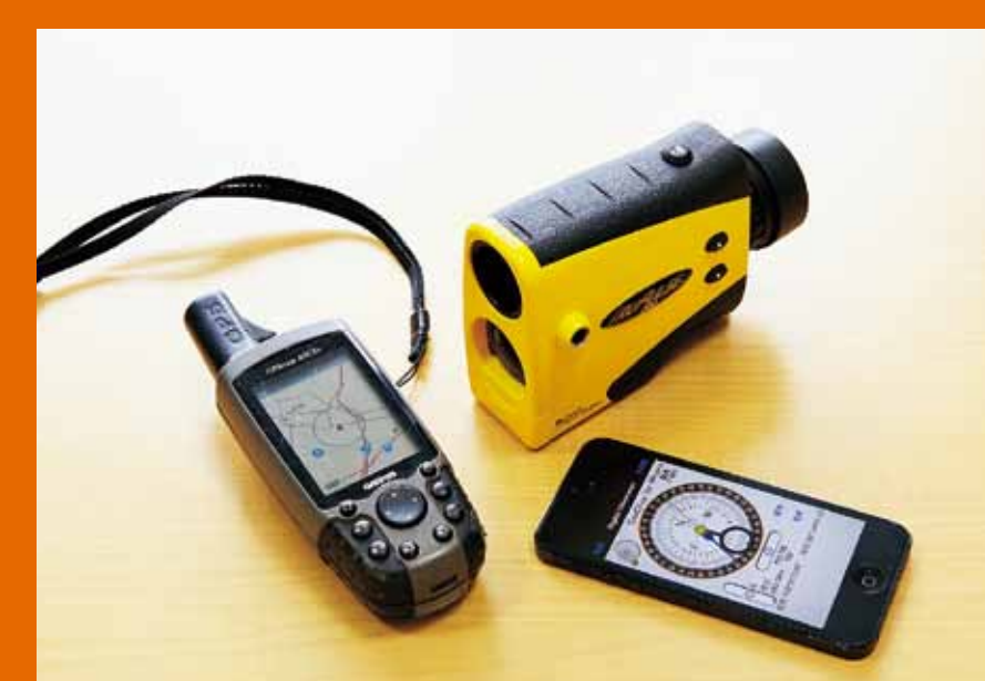
Field devices for disaster study (range finder, GPS and clinometer)
