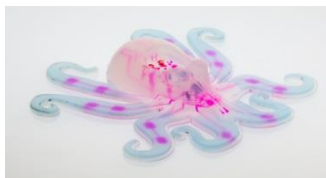
Harvard's Octobot is the first autonomous machine to be made with all soft robotics
